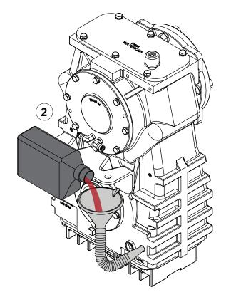
Use the illustrations and instructions to add lubricant to the PTO. Use automatic transmission fluid (ATF) that meets the requirements of DEXRON III or MERCON V.
