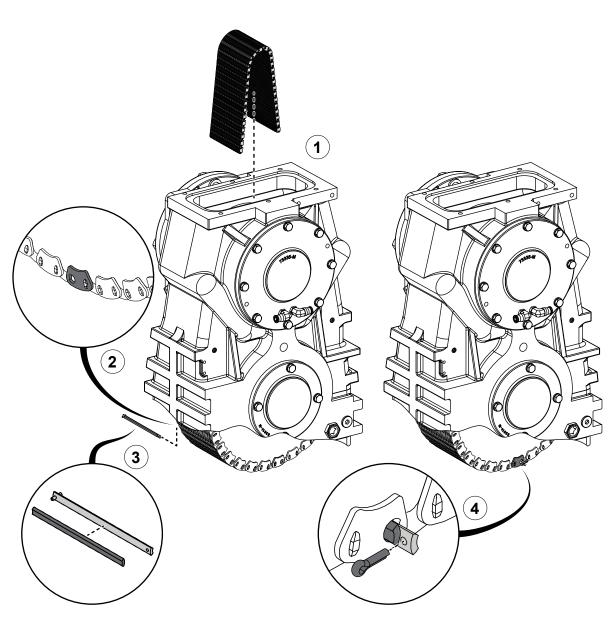
Use the illustrations and instructions to install the drive chain. Replace any components that are worn or damaged.
