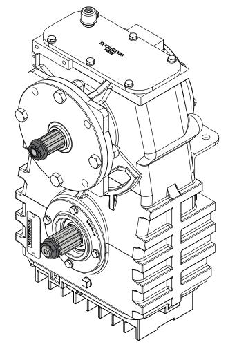
Input and output are on the same side of the case.
