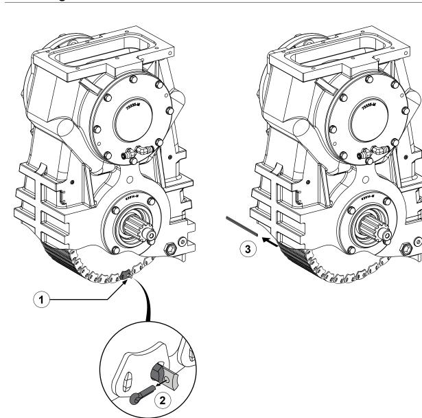
Use the illustrations and instructions to separate and remove the drive chain.
