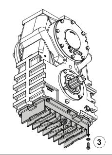
Use the illustrations and instructions to remove the case cover and transmission pan.
