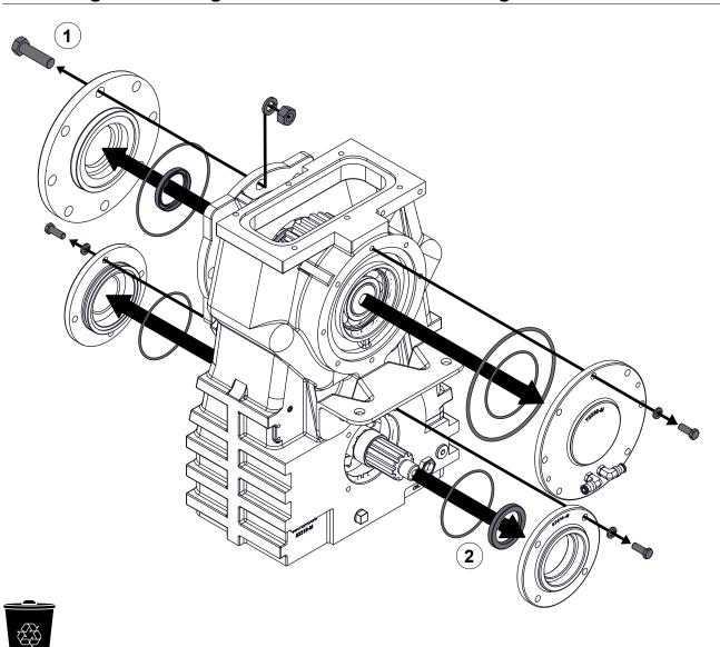
Use the illustration and instructions to remove the bearing covers, oil seal housings, and the associated components.
