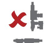
Do not install the dual air primer where the exhaust flow is impeded or where the exhaust flow will damage other components on the apparatus.
