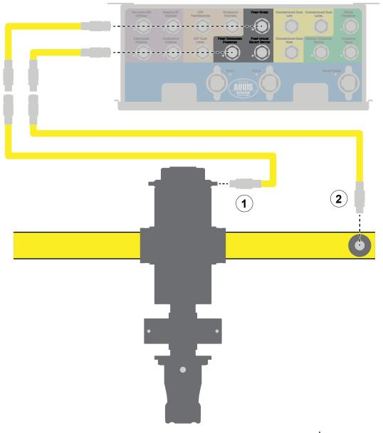
Use the illustration and instructions to connect the concentrate pump speed sensor and concentrate discharge pressure transducer to the control box.
