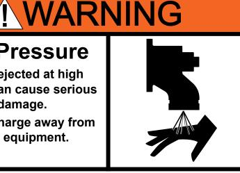
An over-pressure event is an event that causes concentrate to discharge into the on-board tank or external reservoir at a high pressure. Typically two conditions cause over-pressure events: the pressure relief valve is activated or you manually over-prime the system.
