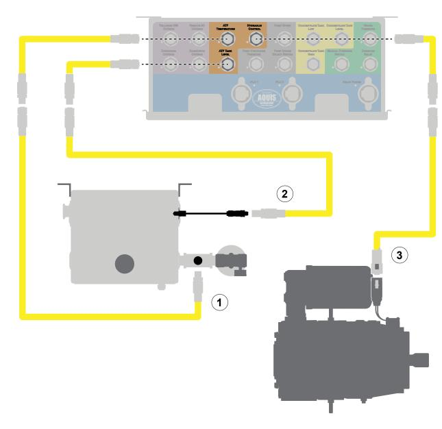
Use the illustration and instructions to connect the hydraulic sensors and hydraulic pump to the control box.
