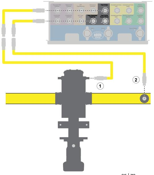
Use the illustration and instructions to connect the concentrate pump speed sensor and concentrate discharge pressure transducer to the control box.
